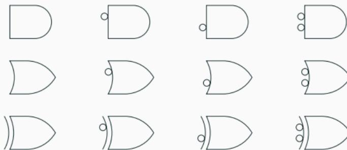
No need for NOT gates: negation is performed on the input of the next gate.
