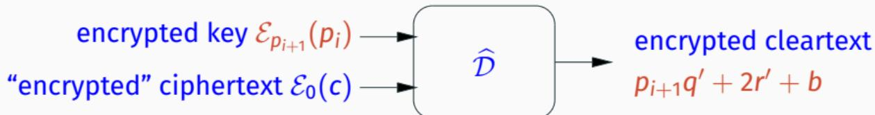
To avoid “circular security” (encrypting a key with itself), we can switch keys at bootstrapping time.
