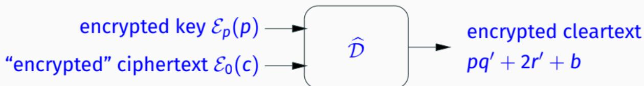
The homomorphic evaluation  $\widehat{\mathcal{D}}$  of the circuit  $\mathcal{D}$  takes as inputs the encrypted private key and the (trivially) encrypted ciphertext  $c$ , and outputs an encryption of the cleartext.
