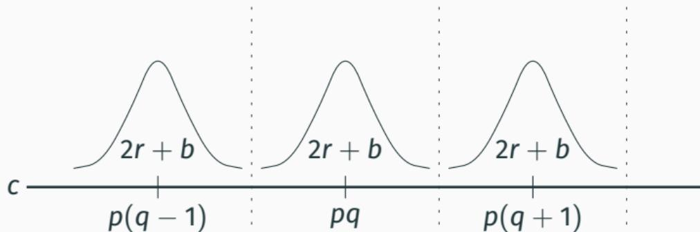
From the ciphertext  $c$  and the private key  $p$ , we recover  $q = \lfloor c/p \rfloor$ , and
